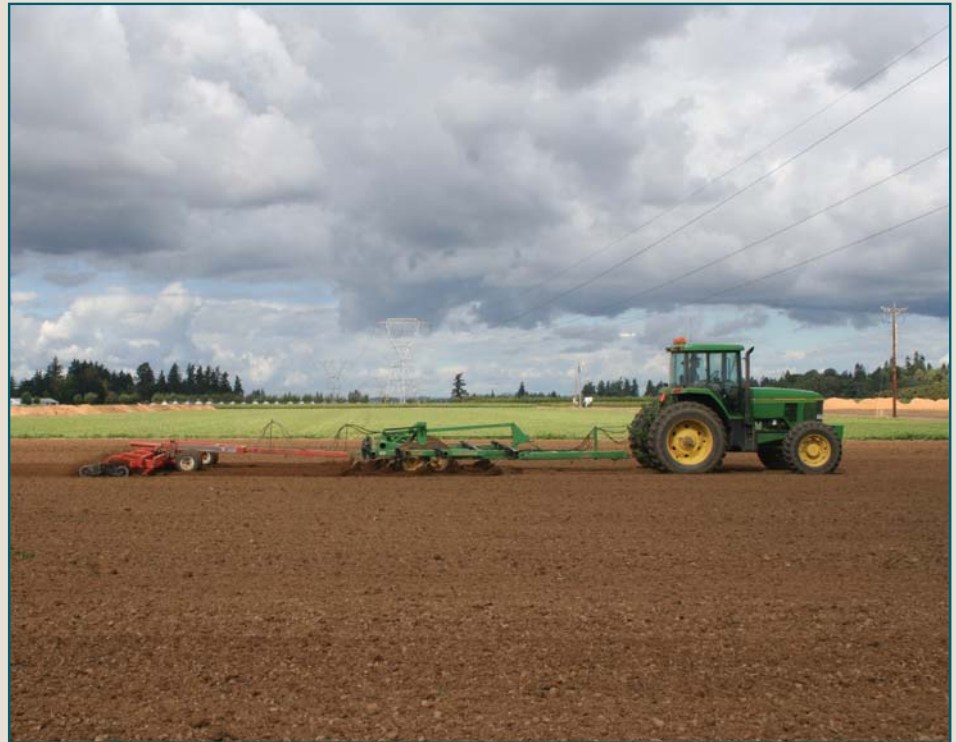
Preparing ground for planting with field cultivator and roller harrow.
