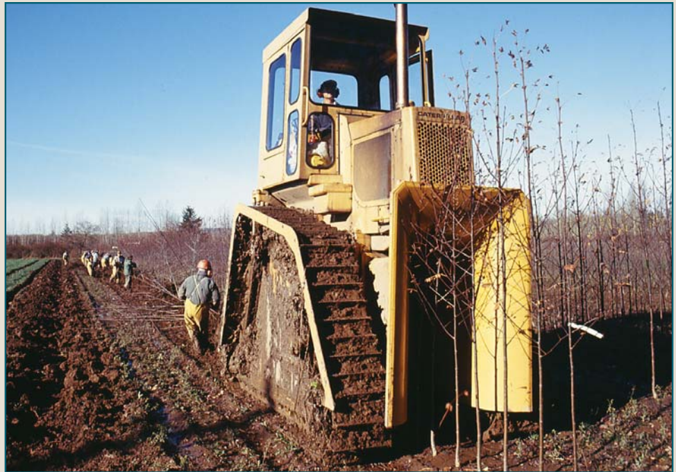
Harvesting trees with D-3 Tree Digger.
